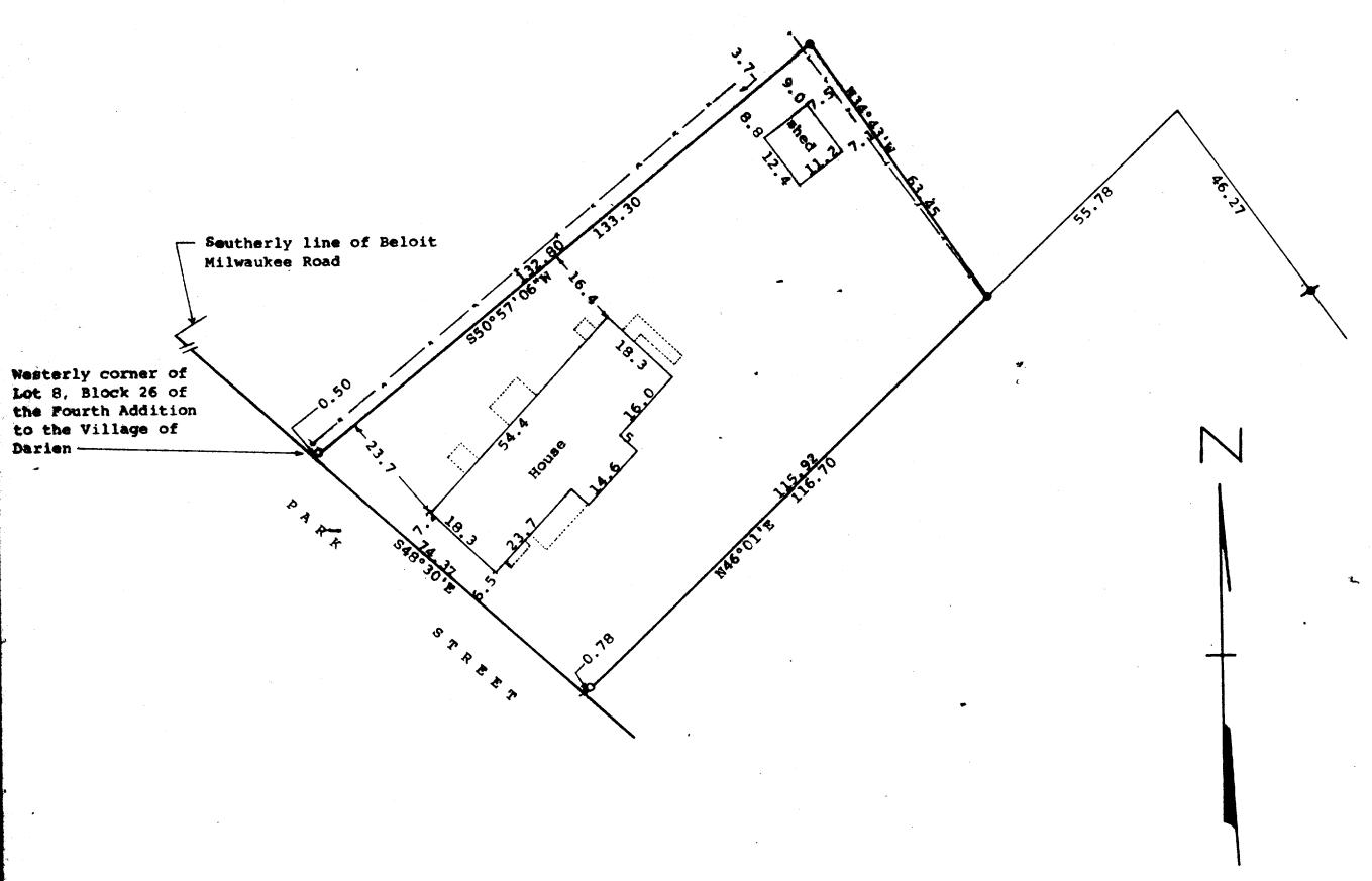
Scale -1" = 20"x = cross in concrete o = 1" Iron Pipe Found 2 = 3/4" Iron Pipe Found •= 1½" X 24" Iron Pipe Set
